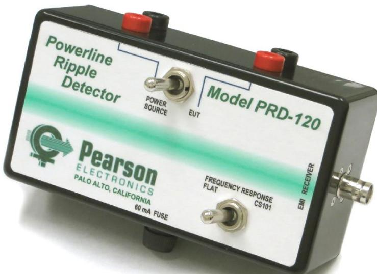
**Description.** The Pearson PRD-120 facilitates the measurement of power line ac ripple using a frequency selective voltmeter, i.e., EMI receiver or spectrum analyzer. In so doing, it greatly simplifies both the manual and automated measurement of injected ripple in such standards as MIL-STD-461 CS01/CS101, RTCA/DO-160 section 18 and MIL-HDBK-704-2 through -6.
