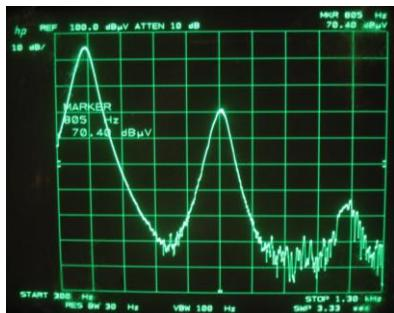
**Figure 3a:** View of 6.3 Vrms 800 Hz ripple on a 400 Hz 115 Vrms bus, using the PRD-120
