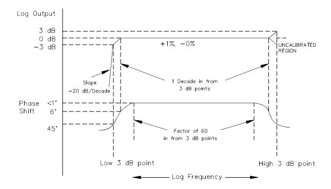
Pearson Current Monitors exhibit amplitude response and phase shift as a function of frequency similar to that depicted in the above figure. To apply this graph to a specific model, use the low and high 3 dB points given in the specification sheet.
